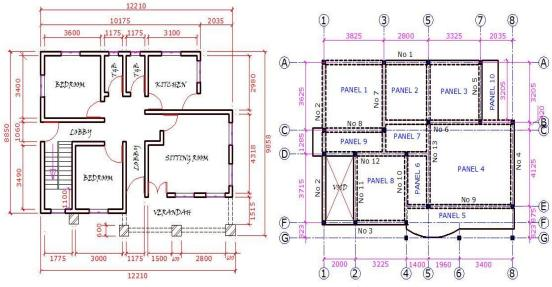
Figure 148: Floor plan and corresponding structural layout Source: Structville.com
