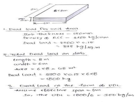
Figure 149: Example of load calculation of a slab Source: Quora.com
