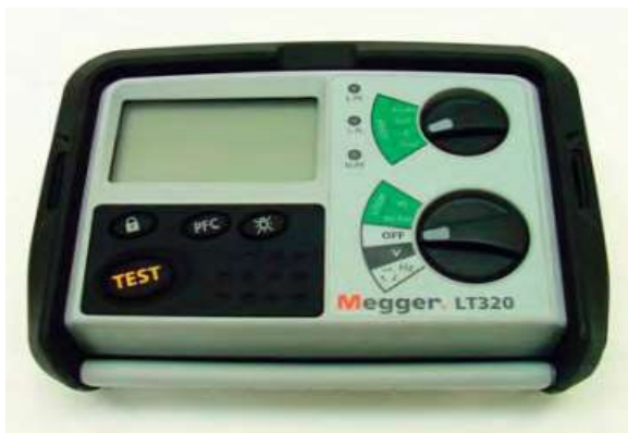
Figure 310 Earth-loop impedance tester
