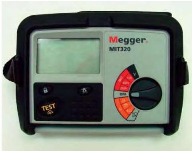
Figure 309 Modern insulation and continuity tester
