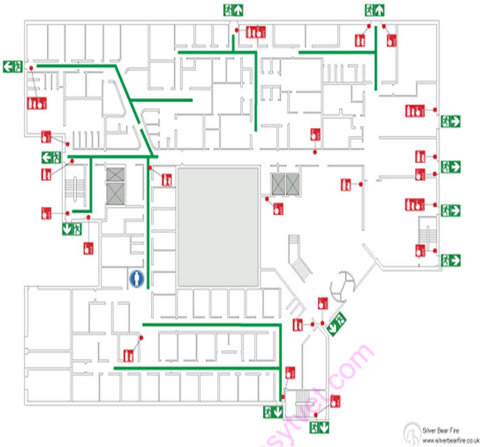
Figure 187 - Fire Control System
