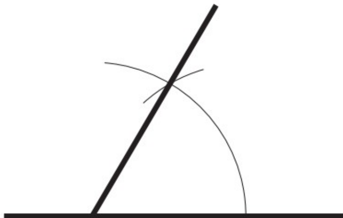
Figure 39 Constructing an angle of 60^\circ
